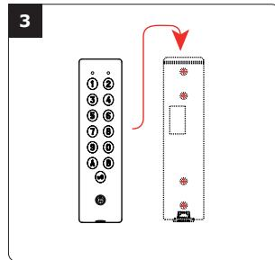
Insert the cable in the hole access area of the back plate. Then mount the keypad on the back plate, placing first the top in the hooks and then the bottom.
