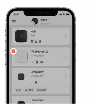
If FireProtect 2 malfunction is detected (for example, there is no connection with the hub), the malfunction counter is displayed in the device field in the Ajax apps.
