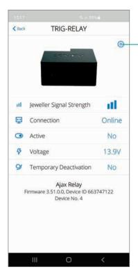
Once the device "TRIG-RELAY" has been selected, the configuration screen will appear. Click on the wheel at the top right
