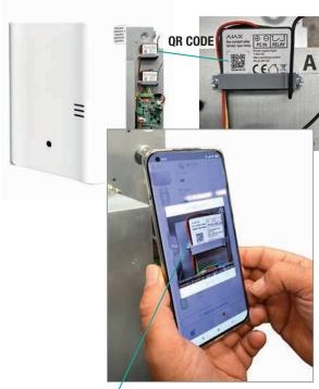
Place the camera of your Smartphone in front of the QR CODE to acquire, automatically, the ID of the relay device
