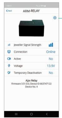
Once the device "ARM-RELAY" has been selected, the configuration screen will appear. Click on the wheel at the top right
